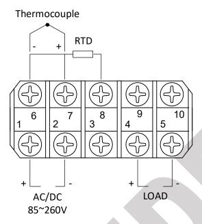
Figure 1 Back Terminals Wiring Diagram
