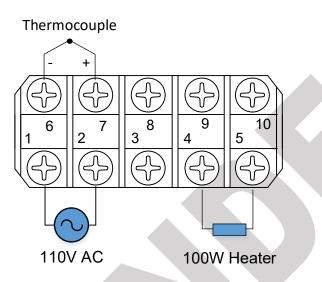
Figure 5. Wiring Diagram
