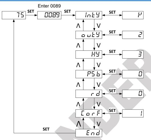
Figure 3. Initial function parameters setup
